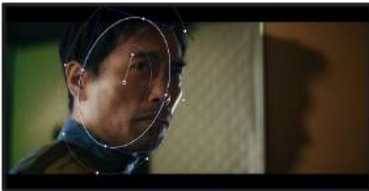
Power windows let you make secondary corrections to specific parts of your image
