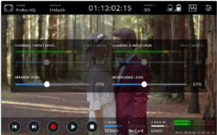
On the 12G video assist, channel inputs will be disabled when no XLR audio is connected
