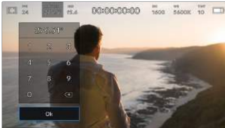
Use the manual shutter keypad to enter your shutter timing of choice when shooting outdoors or under flicker free lights
