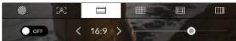
Tap the 'frame guides' icon while accessing 'LCD monitor options' to access your Blackmagic Pocket Cinema Camera 4K's frame guide settings
