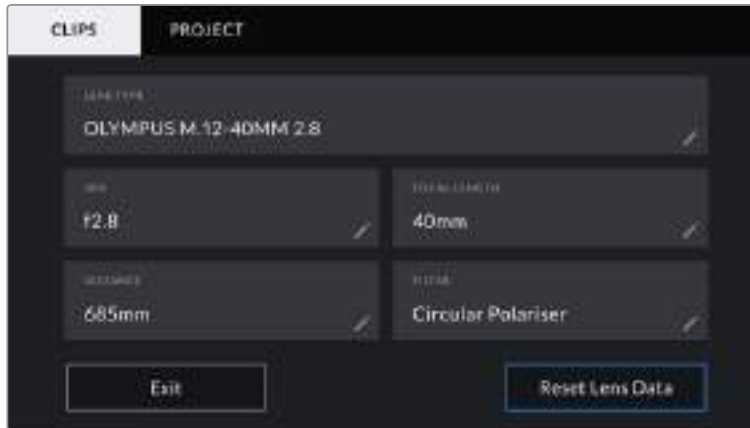
The 'lens data' menu showing information automatically populated from an attached lens, and filter information that has been manually entered
