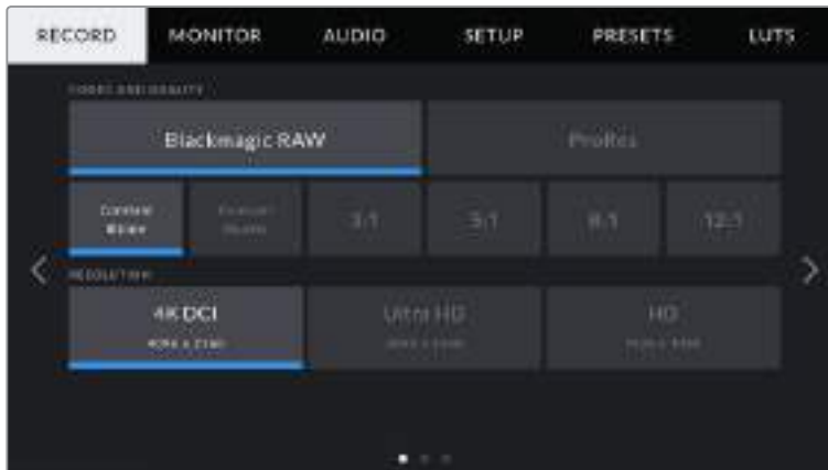
Tap the 'record,' 'monitor,' 'audio,' 'setup,' 'presets,' and 'LUTS' headings to move between your Pocket Cinema Camera 4K's dashboard tabs
