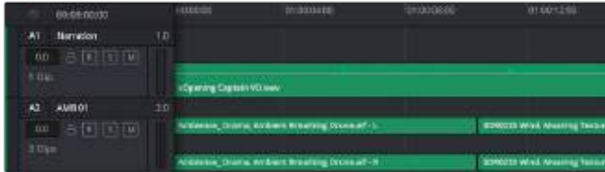
The track header on track A1 indicates a mono track with a single lane for mono audio, and the A2 track header indicates a stereo track with two lanes to accommodate stereo audio
