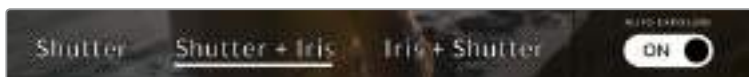
While in the shutter menu, tap 'auto exposure' to access shutter based auto exposure modes
