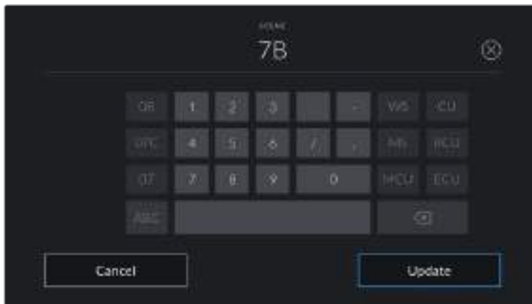
When entering 'scene' metadata, the camera prompts you with scene number suggestions to the left of the touch keyboard, and shot types to the right
