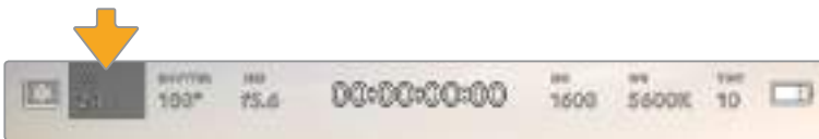
Blackmagic Pocket Cinema Camera 4K's frames per second indicator. Tap this to access frame rate settings
